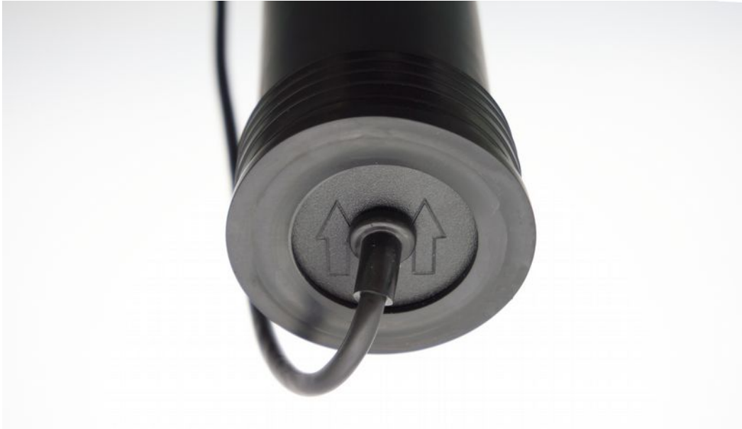
Figure 9.2: Add additional marks to the Super Sensor aids in the scan.
