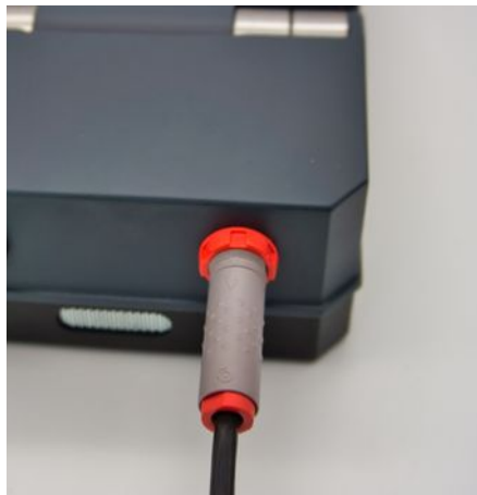
Figure 6.2: Connection of Power Pack
