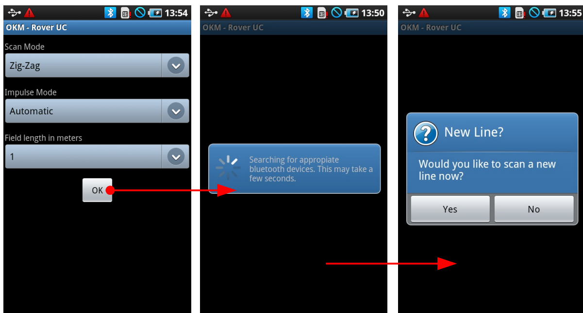
Figure 7.5: Establishing a Bluetooth connection in operating mode "3D Ground Scan"
