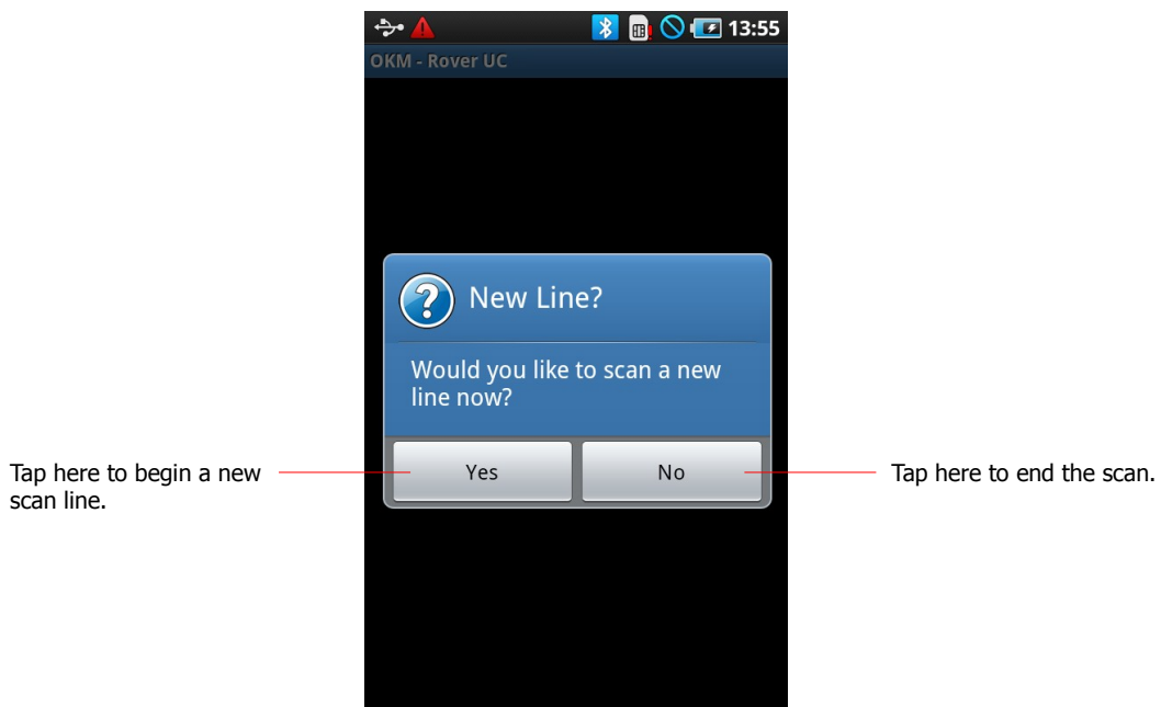
Figure 10.3: Starting a new scan line
