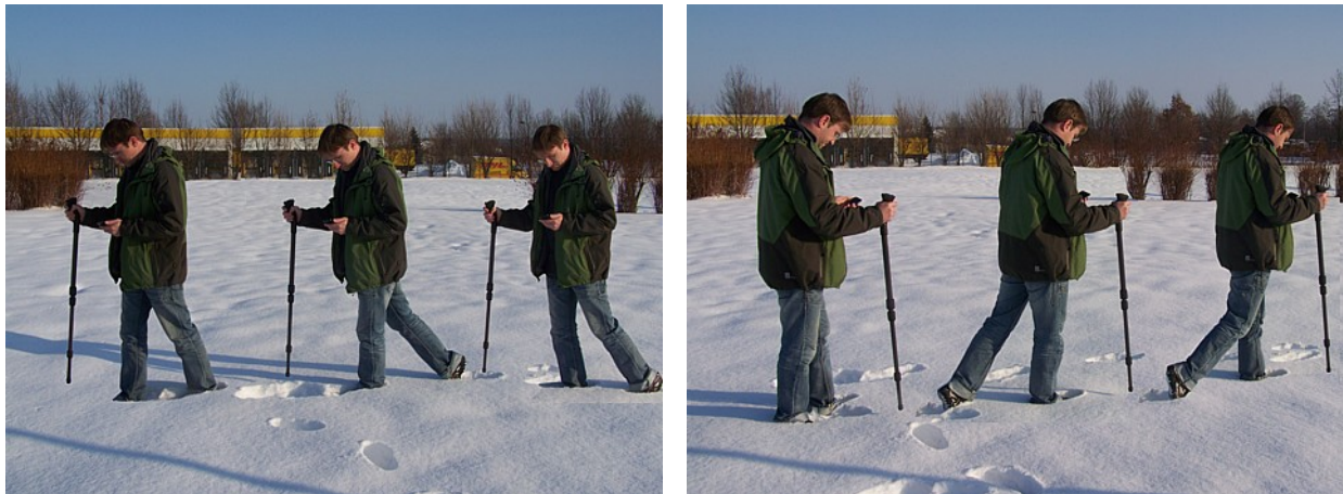
Figure 7.6: "Zig-Zag" scan in operating mode "3D Ground Scan"
