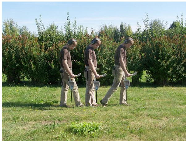
Figure 7.2: Probe should point always to the down and should not be turned
