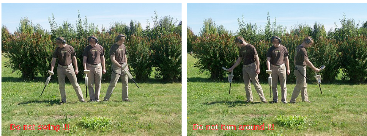
Figure 7.3: Pivoting or turning of the probe falsifies the measurement
