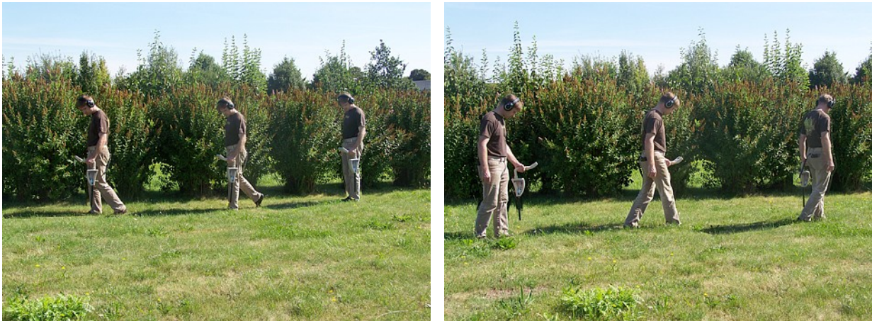
Figure 7.5: "Zig-Zag" scanning in mode Ground Scan
