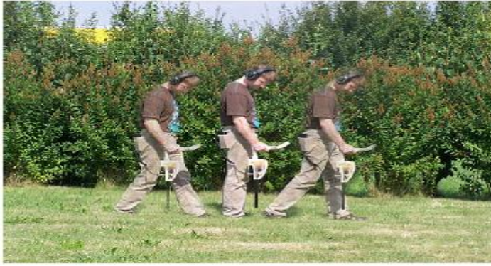
Figure 7.2: Probe should point always to the down and should not be turned
