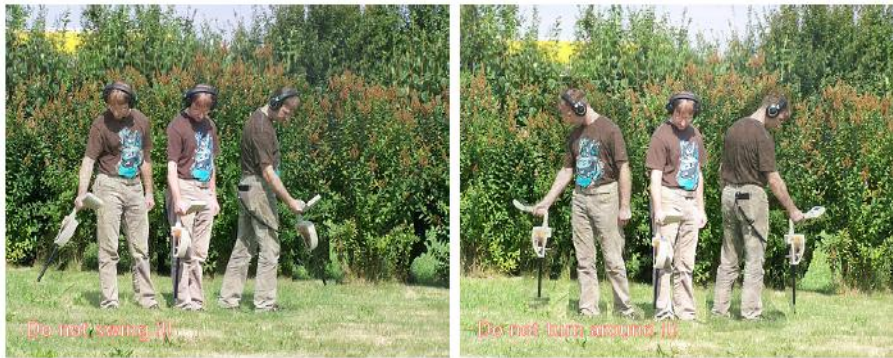
Figure 7.3: Pivoting or turning of the probe falsifies the measurement
