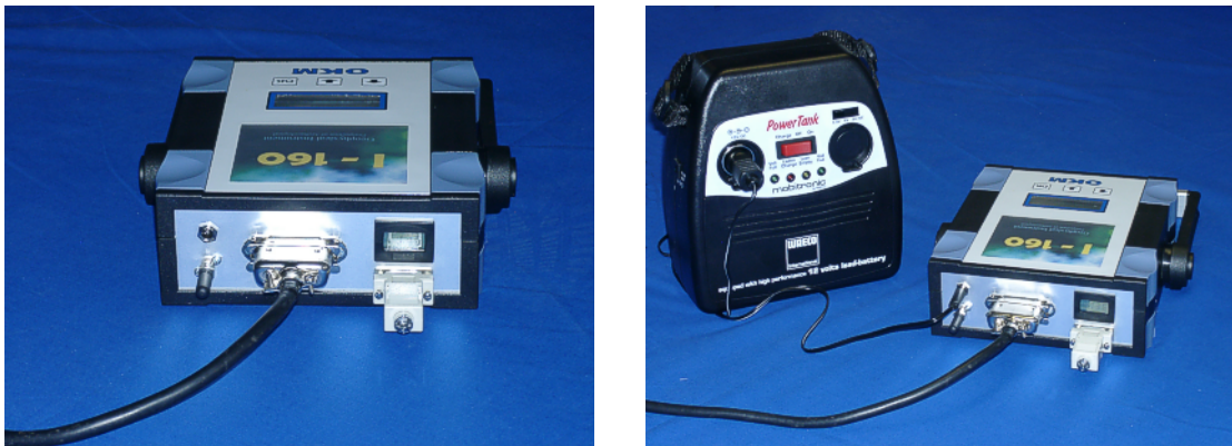
Figure 3: Connection of Control Chip and External Power Supply
