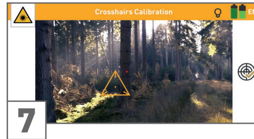
7 Before proceeding with the measurement, you may recalibrate the crosshairs position – see 4.6 Set Crosshairs Position on page 17 – and the Bionic Sensors – see 5.4.1 Calibrate Bionic Sensors on page 24.
