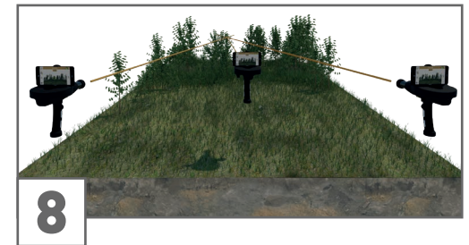
8 As soon as you get a hit on the same target spot, it is likely it is a potential target. You may perform further control scans to verify the target spot.
