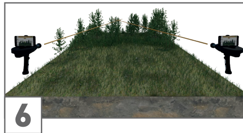
6 Perform a Control Scan from a different direction at about 80 to 1600 ft (25 to 500 m) distance from your first spot.
